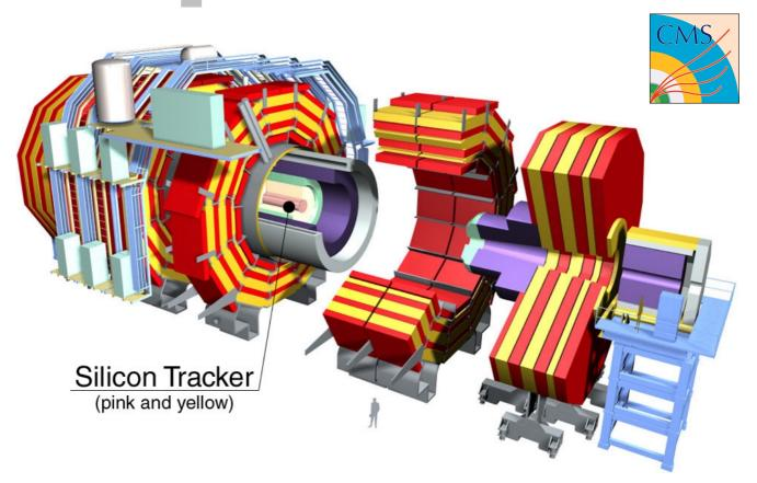
Tracker Silicon strip and pixel detectors (206m<sup>2</sup>)
