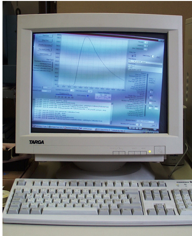
Figure 5.44: Image of a CRT monitor, located approximately 2 m away from the magnet coil with an inner flux density of 10 T. The magnetic field not only rotates the picture geometry, but also disturbs the color representation.
